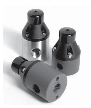
**Griffco M-Series** diaphragm pressure relief valves are designed to protect chemical feed systems from over pressure damage caused by defective equipment or a blockage in the chemical feed line. Robust construction ensures reliability in the rigorous service of municipal and industrial applications. Wetted materials include: **PVC, CPVC, PP, PVDF, PTFE, Halar, 316 SS, A20 and Hastalloy C.** Available sizes: 1/4" - 1/2".
