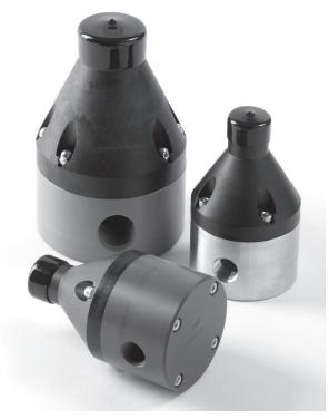
**Griffco** high flow diaphragm pressure relief valves are designed to protect chemical transfer systems from over pressure damage caused by defective equipment or a blockage in the chemical line. Large orifice sizes facilitate high flows and high viscosity. Wetted materials include **PVC**, **CPVC**, **PP**, **PVDF**, **PTFE**, **316SS**, **A20** and **Hast**. **C**. Available sizes: 1/2", 3/4, and 1".
