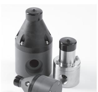
**Griffco G-Series** diaphragm back pressure valves are designed to enhance the performance of chemical feed systems by applying a continuous back pressure to the chemical feed pump, while also acting as an anti-syphon valve. Robust construction ensures reliability in the rigorous service of municipal and industrial applications. Wetted materials include: **PVC**, **CPVC**, **PP**, **PVDF**, **PTFE**, **Halar**, **316 SS**, **A20** and **Hast**. **C**. Available sizes: 1/2" - 4".
