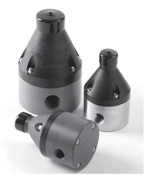
**Griffco** high flow diaphragm back pressure valves are designed to enhance the performance of higher flow, continuos feed pumps that require a constant head pressure, while also acting as an anti-syphon valve. Larger orifice sizes make the valve ideal for use with higher viscosity fluids. Wetted materials include: **PVC**, **CPVC**, **PP**, **PVDF**, **PTFE**, **316 SS**, **A 20 and Hast. C**. Available in ½", ¾" and 1" sizes.
