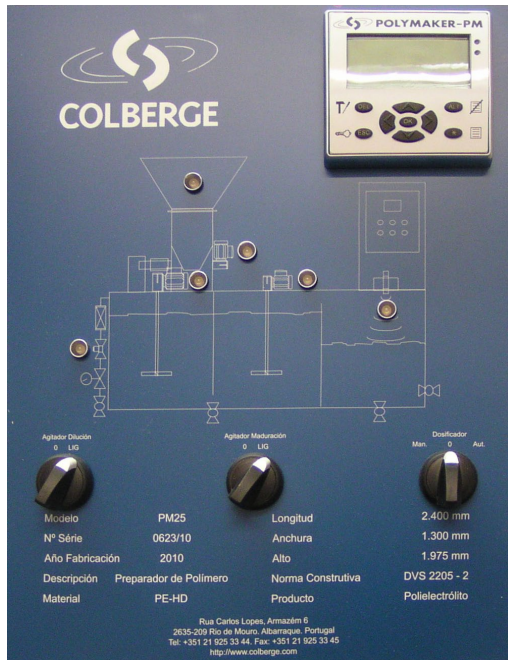
Process control panel of the prepurer
