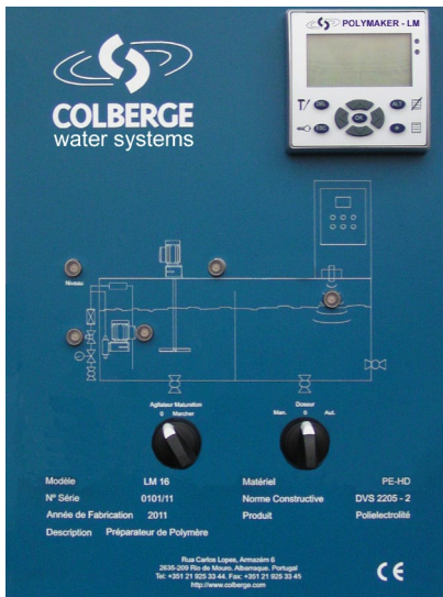
Process control panel of the preparer
